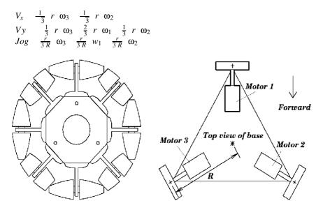
We observe that if  $\omega_3 = \omega_2$  and  $\omega_1 = 0$  then  $V_x = 1.15 \ r = \omega_3$  that is greater than the velocity which could be achieved by a unicycle robot.
