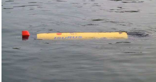
Figure 6.8: Autonomous Underwater Vehicle used in the PISCIS project at Porto University.
